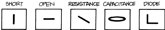
Figure 27. X-Y COMPONENT CHECKING requires the transistor checker shown above. With it connected to your scope and the scope in the X-Y mode, patterns like those illustrated indicate the component's condition. The waveforms shown are found when the components are not in a circuit; in-circuit component patterns will differ because of resistors and capacitors associated with the component.
